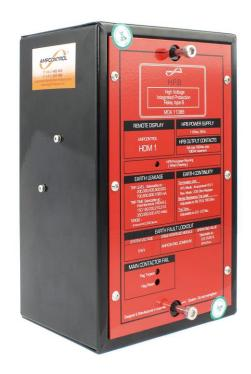
The HPB Relay has 5 digital inputs, which feed into a microprocessor unit. The microprocessor has been programmed to control three output relays. Relay MCR for the main contactor and Relay CBR for the circuit breaker. RL3 is used to control the supply to the Cable Connection Module enabling it to perform the Earth Fault Lockout test. All of the tripping logic and outlet control is performed by the microprocessor, so that only minimal external control is required.
